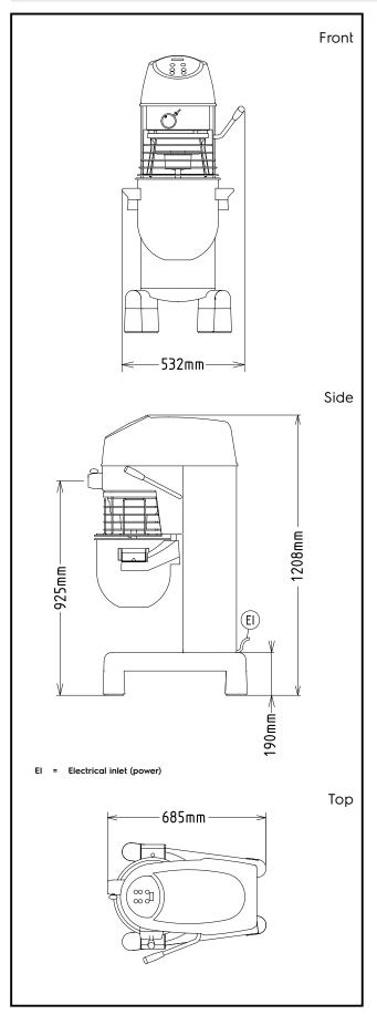
Electric Supply voltage: 200-240 V/1N ph/50/60 Hz Electrical power max.: 1.01 kW Capacity: Performance (up to): 6 kg/Cycle
